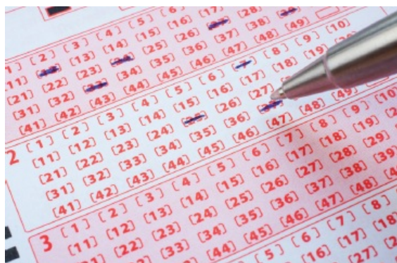
Figure 2.4: A typical input sheet for an OMR reader.
