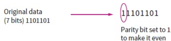
Figure 9.10: Creating an even parity.
