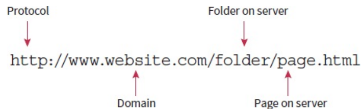
Figure 9.15: The component parts of a URL
