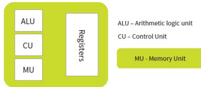
Figure 1.3: Overview of a processor.
