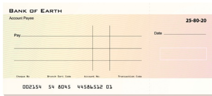
Figure 2.6: A standard bank cheque; notice the number in electronic ink along the bottom.
