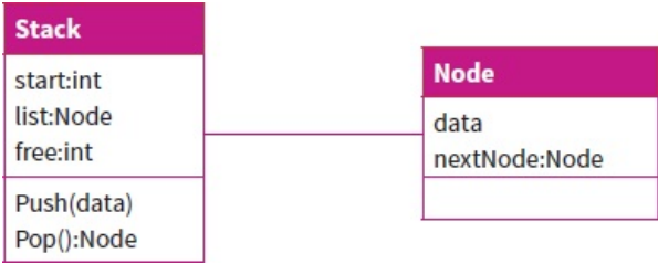
Figure 6.2: Class diagram for stack.
