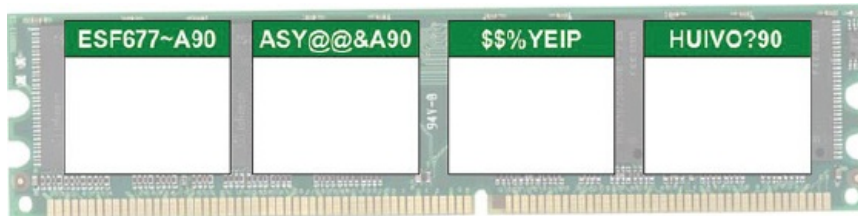
Figure 20.19: Storage locations in a computer's memory.
